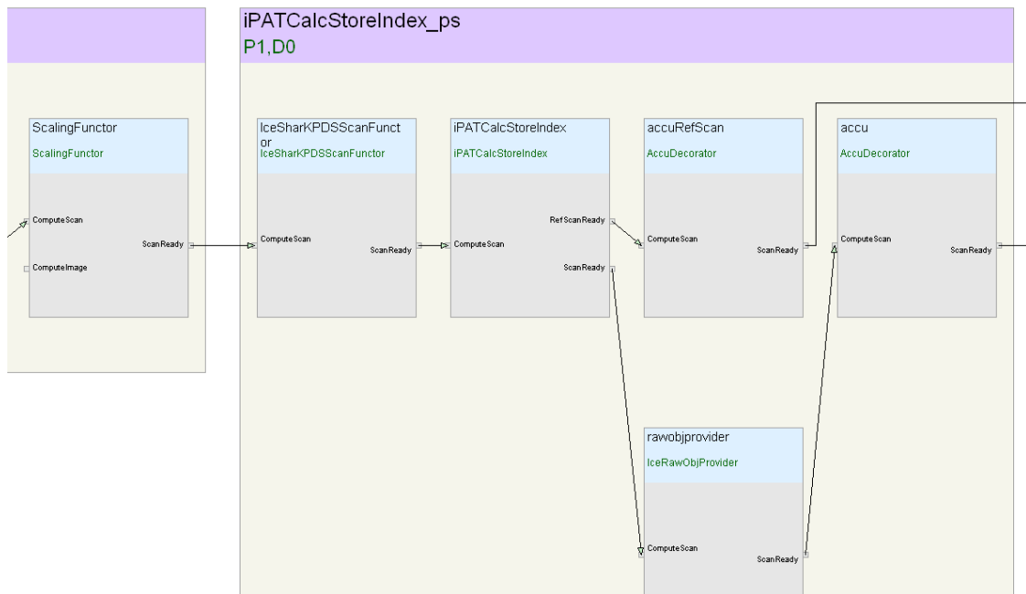
Figure 5.4 Ice Pipeline for image reconstruction. The added IceSharkPDSScanFuncion saves k-space from the angiographic data in the Parc Data Storage (PDS) and retrieves it when a partial Shark is acquired for the LGE reconstruction.
